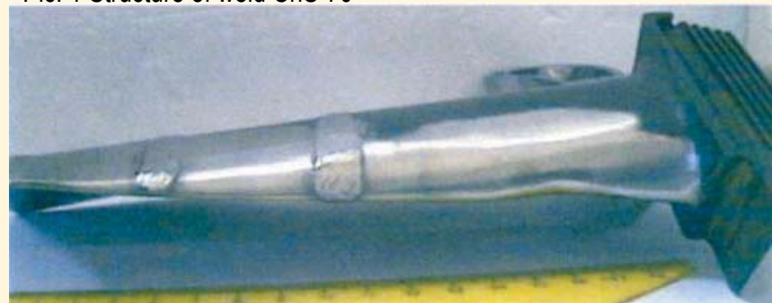
Pic2. Repair welding on blade of alloy EP 539
