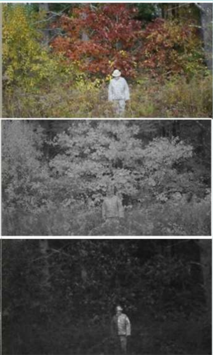
Visible, IR, UV images of uniform with right side treated with UVRC-A 7%
