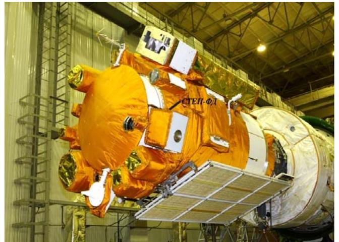
Pic.2. Flight model of the STEP-F device in the set of complex scientific apparatus "Photon" before transportation to the start platform.
