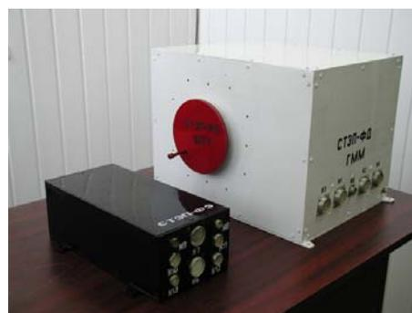
Pic.5. Dimensional model of the STEP-F device
