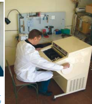
Fig.2. Microtome-cryostat for the express diagnostics of oncological diseases in interoperation conditions.
