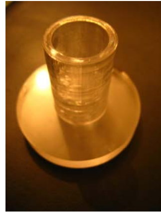
Fig. 1. A single-piece sapphire preform for the gyroscopic resonator (before any processing)
