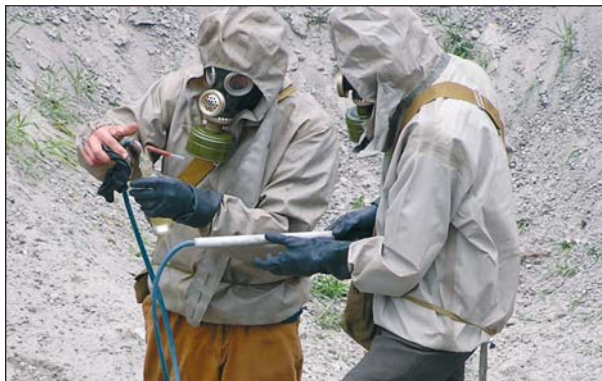
Assessment of contamination after Open Burning Open Detonation (OBOD) Technology of PFM-1 Destruction
